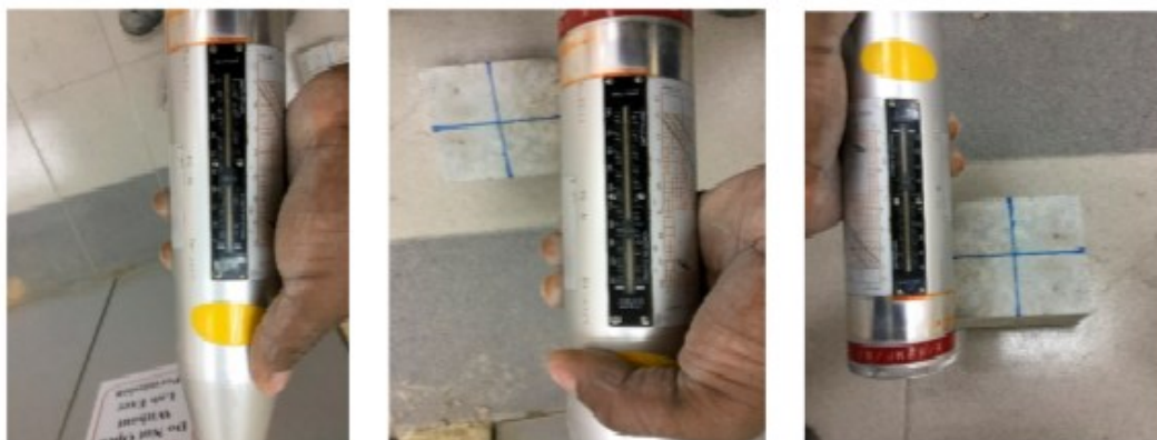
Figure 3.0: Rebound hammer reading after testing on concrete sample using rebound hammer method
